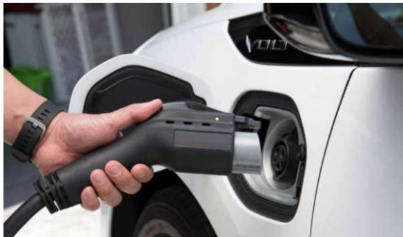
Step 1: Plug in the charging interface
