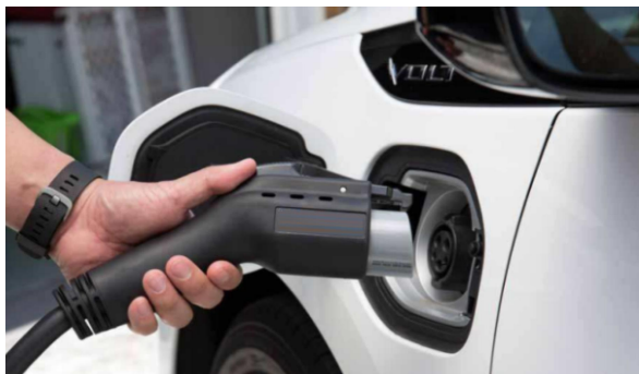
Step 1: Plug in the charging interface
